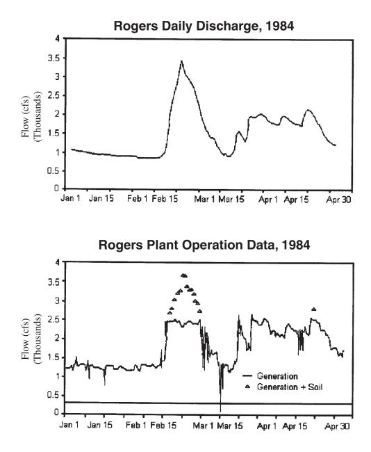
Figure 4.–Daily discharge at the USGS gauge at Evart (top figure), compared with total flow at the Rogers Project (bottom figure), 1984, Muskegon River, Michigan. Figure from Lawler, Matusky & Skelly Engineers (1991a).
