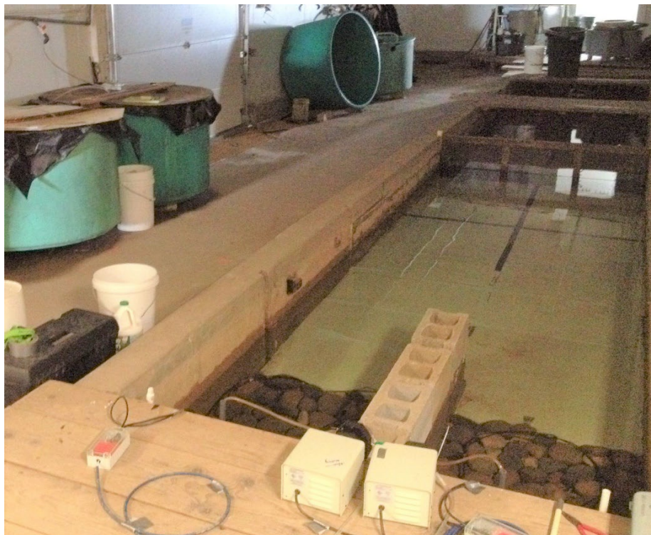
FIGURE 2. One of two replicate flumes used for water choice experiments in 2019. Top image (looking upstream) shows areas where odors were applied, and bottom image looks downstream. Small boxes at upstream end are dosing pumps for applying odors and round tanks on left held Walleyes. All trials occurred at night with all lights off.
