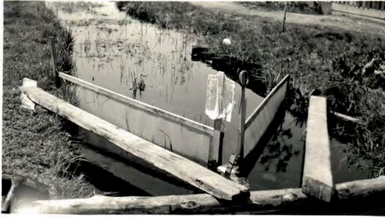
Front view (looking upstream) of pike fry trap on Peterson's ditch. Note vegetation in ditch.
