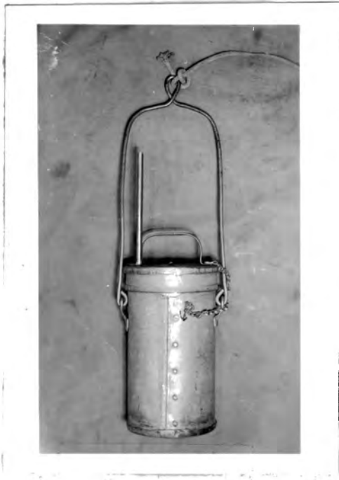
Figure 11. Water sampler, used in obtaining samples for chemical analysis.
