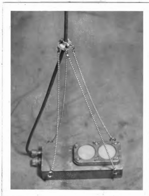
Figure 14. Target of photometer, showing method of suspension by electric cable.
