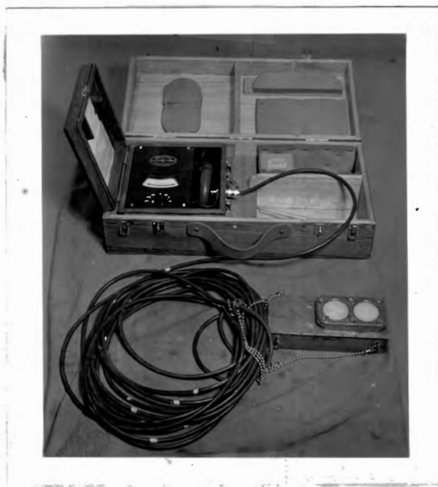
Figure 13. Submerged photometer, with cable and microammeter.
