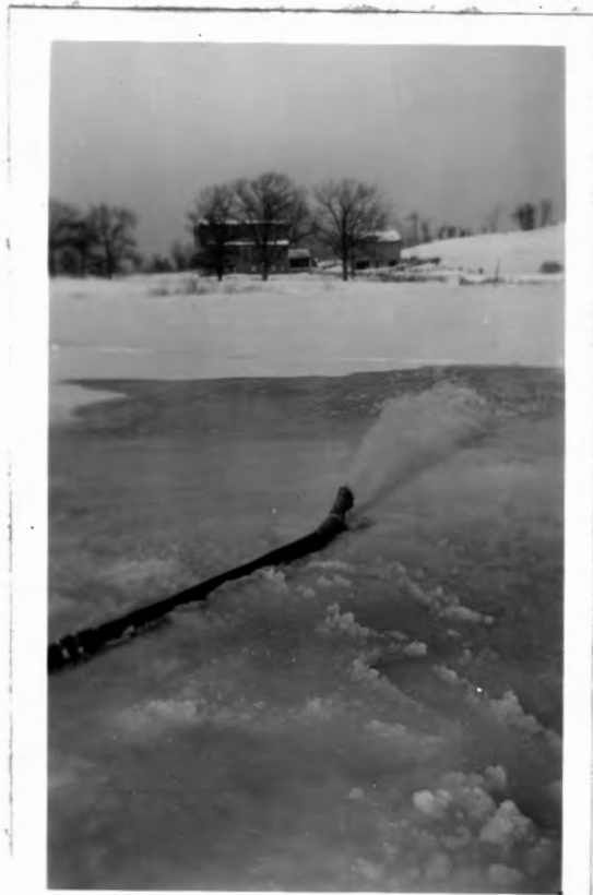
Figure 7. Discharge through open end of hose.
