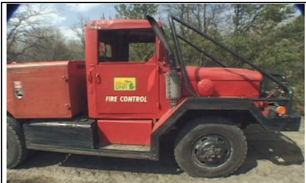
The bumper and fuel tank guard are fastened to the frame. The fender guard connects between them. The grill guard and limb risers sit on top of the bumper and fender guard.
