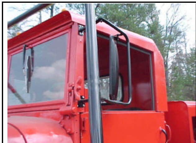
The mirrors can be hidden behind the limb risers by changing the hinge point.
