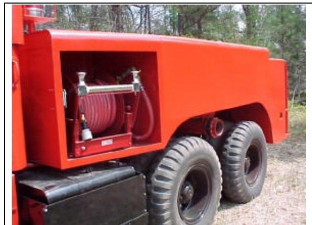
Figure 1 - Left side view showing front hose reel and tank dump (between wheels).
