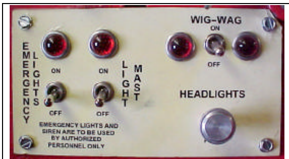
Figure 2 - Dash Panel with Toggle Switches
