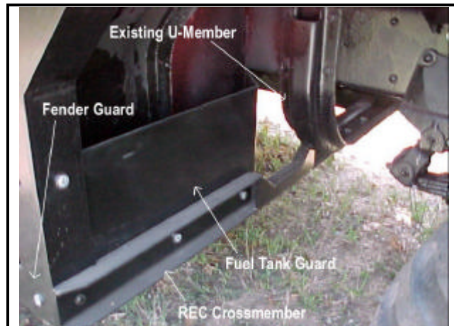
The crossmember attaches to the 5-Ton's U-shaped frame crossmember.
