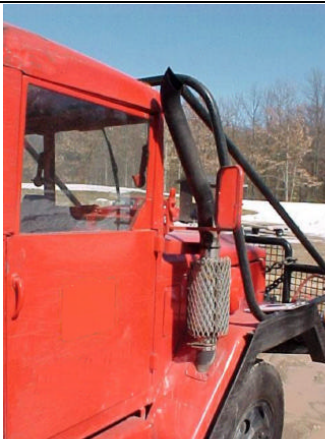
The exhaust stack is rerouted behind the limb risers for protection.
