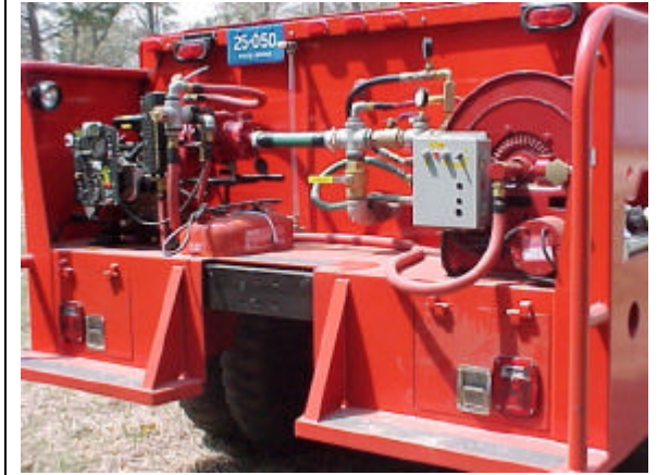
Figure 3 - The pump deck at the rear has room for an auxiliary pump, hose reel, and proportioning system, if desired. Two compartments add storage behind the wheels.
