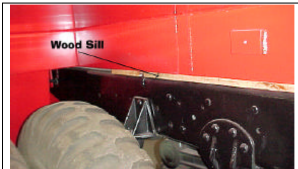
Figure 5 - The tank rides on a 3/4 inch hardwood board to prevent metal-to-metal wear.
