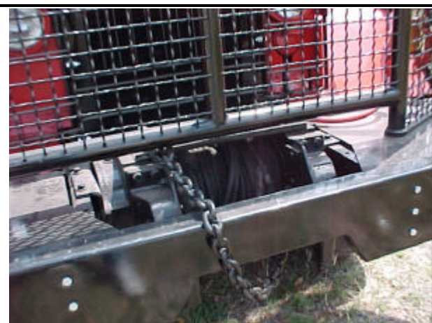
The REC bumper accommodates trucks with or without a winch.
