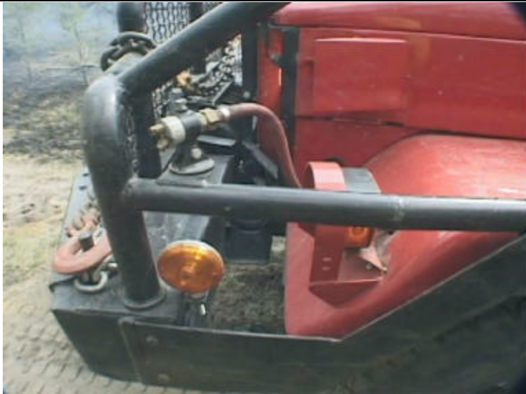
The fender guard is connected to the bumper. In combination with the grill guard, they protect the cab sheet metal.
