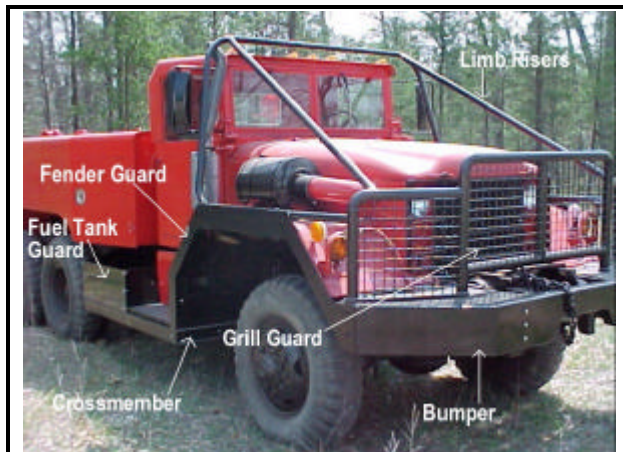
The major parts of the REC brush protection design.
