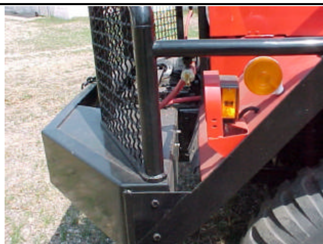
The fender grill guards bolt to the bumper.
