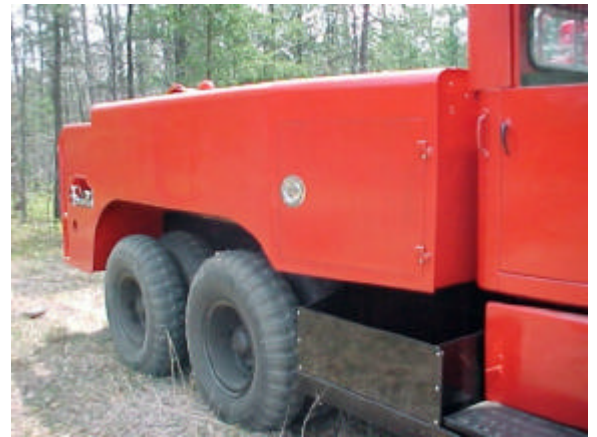
Figure 2 - Right side showing front compartment door and right rear hose reel opening.
