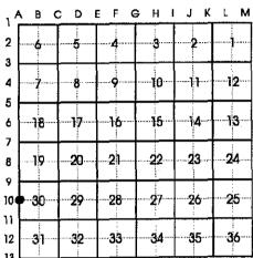
Description of corner evidence found and/or method applied in restoring or reestablishing corner: A-10 Found 3/4"x24" iron in monument box 0.08' West of the East line of Section 25, Town 4 North, Range 15 West Iron in monument box North rec. = 30.16 meas. = 30.33
