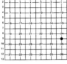
DEKEYSER 1980 1" PIPE ON CENTERLINE ROAD TWIN 12" CHERRY S05°E 24.90' TWIN 12" OAK N50°E 89.50' U-POLE N80°W 97.38'
