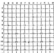
B. Description of corner evidence found and/or method applied in restoring or reestablishing corner: Traversed between G-9 and G-11 and set witness corners on section line on North and South shores of lake.
