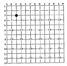
Description of original monument and accessories and/or subsequent restoration: Original corner established by Austin Burt on June 4, 1851. Set post. Original bearing trees: S 480 W 8 links ( 5.28') 26# E1m
