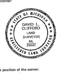
C. Description of monument for corner and accessories established to perpetuate locating the position of the corner: 3/4" Iron Pipe and PA 345 Cap PS #25837, 5' South of centerline East-West ditch and 20' East of North-South ditch.
