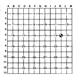
B. Description of corner evidence found and/or method applied in restoring or reestablishing corner: Found Stone with notch in top at surface.
