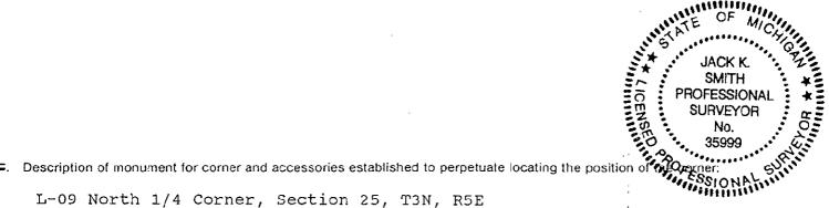
L-09 North 1/4 Corner, Section 25, T3N, R5E Set 36" x 1 1/4" iron pipe with brass cap marked as "Livingston County Monument Corner" N67°W 36" x 1" pipe with brass cap 57.631 36" x 1" pipe with brass cap N73°E 55.75'
