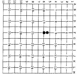
(F6) Center of Section 16. Not established in the original survey. Established and monumented in 1993 by Ronald Bischer RLS 22428. (5-Sec. 16) North 1/16 corner. Not established in the original survey. Established and monumented in 1993 by Ronald Bischer RLS 22428 midway and on a straight line between 1/4 corner and Center of Section.
