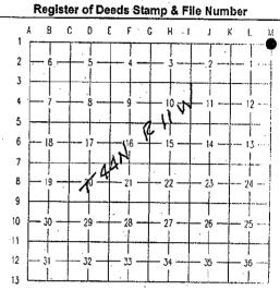
A. Description of original monument and accessories and/or subsequent restoration: (M-1) Township Corner Common to Townships T45N-R11W, T45N-R10W, T44N-R11W and T44N-R10W
