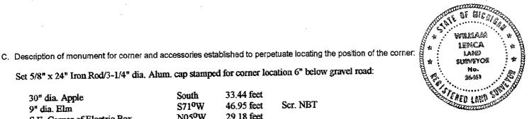
NOTE: All bearings are magnetic bearings. All distances are measured with steel tape. Distances to trees are to nail in side of tree.
