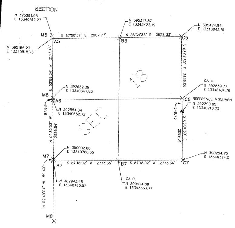
NOTE: DISTANCES ARE MEASURED AT GROUND AND COORDINATES ARE ON GRID
