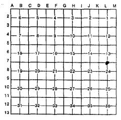
L-7 1/4 CORNER COMMON TO SECTIONS 13 AND 24 LEAVITT TWP; T15N, R15W
