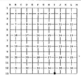
A. Description of original monument and accessories and/or subsequent restoration; (I-13) Standard Corner Common to Sections 34 & 35, T51N, R37W Corner is on the 5<sup>th</sup> Correction Line.
