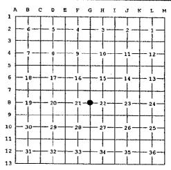
A. Description of original monument and accessories and/or subsequent restoration: (G-8) 1/4 Corner of Sections 21 & 22, T51N, R40W
